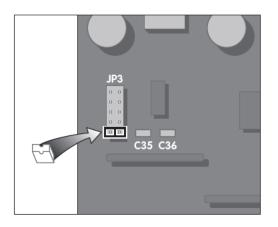
To enable the Auto-Open feature : Use the "jumper" provided and place it on the pinheader of JP3, on the terminals close to C35 as the illustration indicates.
