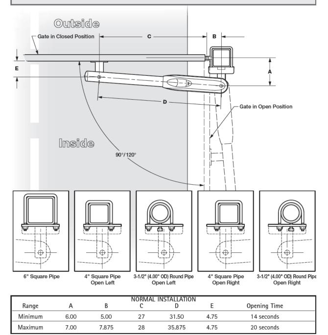
Figure A Open Inside Plan of Installation
