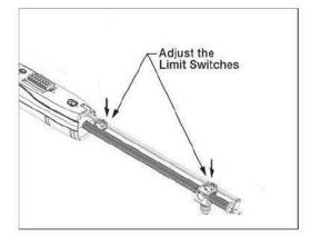
Note: Leave cover off until after the installation of the control box and the electrical installation. Verify that the operator opens and closes to the desired position under power. Make any adjustments as necessary.
