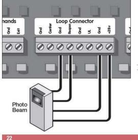
As an alternative to the Outside Reopen Loop, a photo beam unit can be used as shown.
