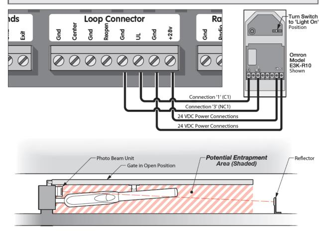
One or more non-contact sensors should be located where the risk of entrapment or obstruction exists, such as the perimeter reachable by a moving gate or barrier.
