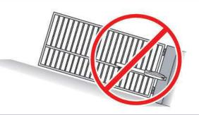
Do NOT Install the gate operator to lift gates
