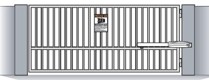
All Warning Signs and Placards must be installed where visible in the area of the gate. A minimum of two placards must be installed. A placard is to be installed in the area of each side of the gate and be visible.
