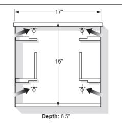
3. Position the ECU Box and secure it to the mounting surface using the Sealed Washers provided (place the rubber side of the washers against the inside of the control box).
