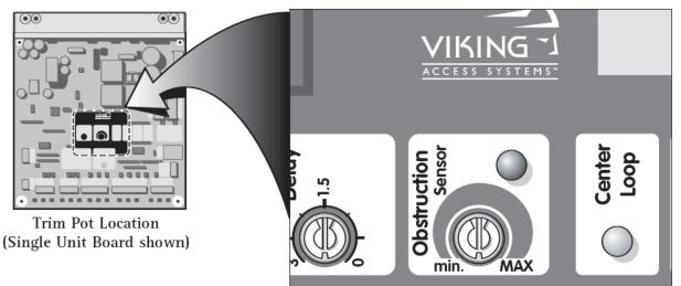
The Obstruction Sensor detects obstructions in the path of the traveling gate. The Trim Pot for the Obstruction Sensor adjusts the sensitivity level that triggers the Sensor.
